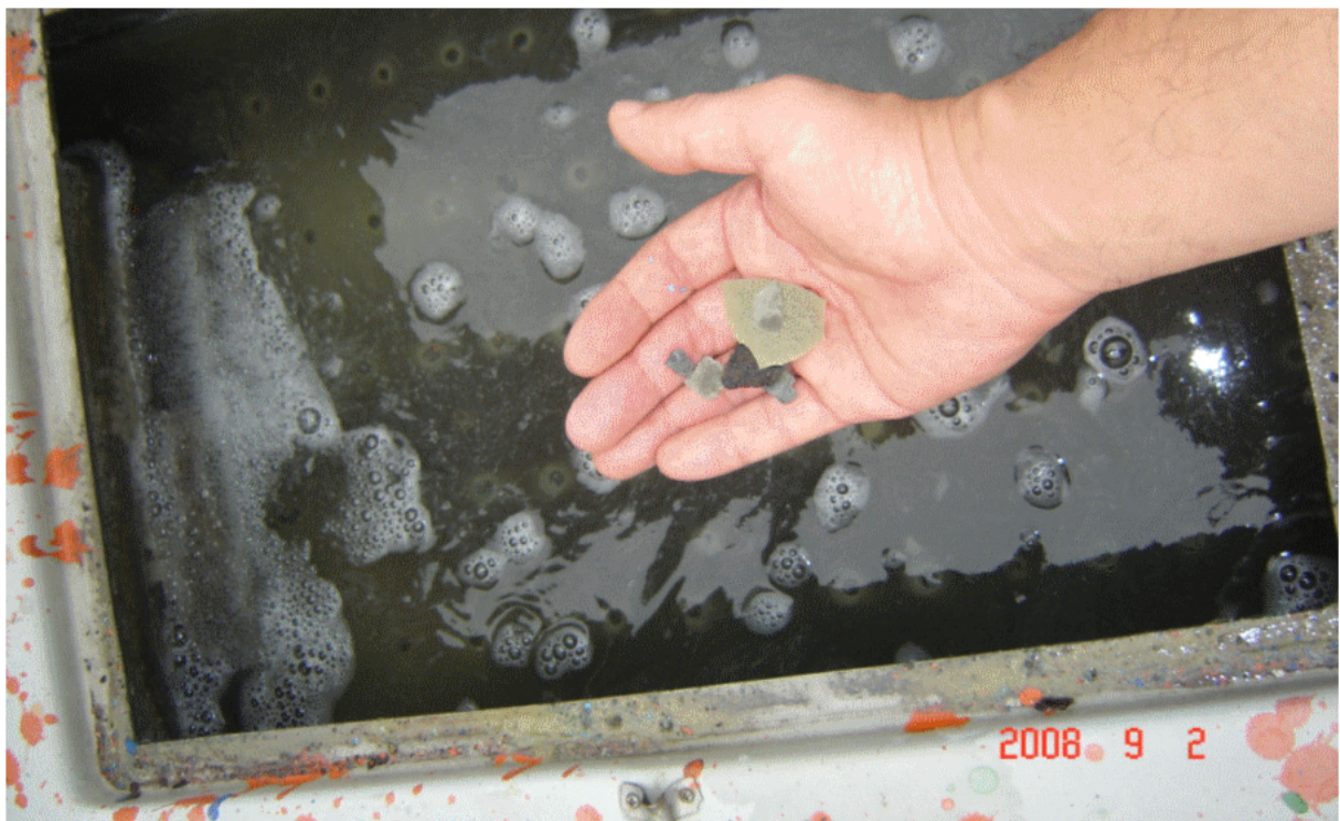
9/2: After 1 week use MB, water in divider start to be clear and less bubble, some scales dropped.
